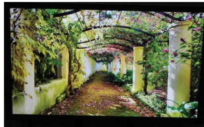
Sharp's 31.5-in. LCD panel relies on an IGZO metal-oxide backplane to deliver 4K resolution
