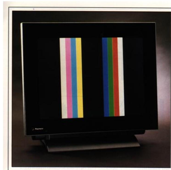
Fig. 3: Plasmaco surprised SID '94 attendees with its first color display. Completed just a couple of hours before the end of the show, the panel displayed a hard-wired pattern of color bars.
