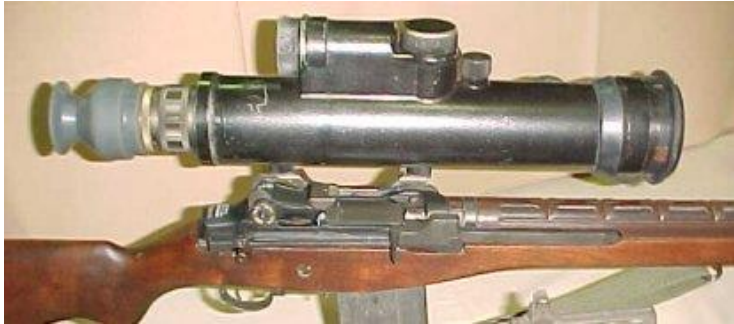
1965-70: AN/PVS-1 Night Vision Sight “Starlight Scope” (gen. 1)
