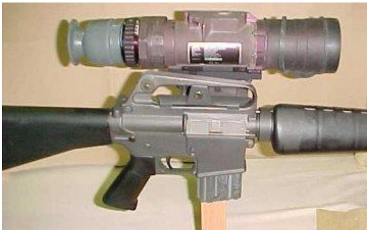
1970-80: AN/PVS-3A Night Vision Sight “Miniscope- Starlight Scope” (gen. 2)
