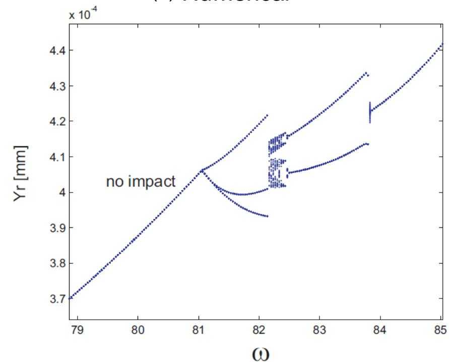
(a) Experimental and (b) theoretical bifurcation diagrams. The following sequence can be identified: no impact (period-1), impact (period-3), impact (period-2), impact (period-1).
