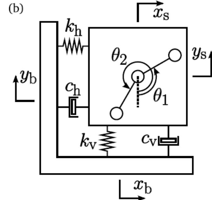
$$\theta_i : m_i l_i \ddot{\theta}_i + c_i l_i \dot{\theta}_i + m_i g \sin \theta_i = -m_i \ddot{x}_s \cos \theta_i - m_i \ddot{y}_s \sin \theta_i, \quad (i = 1, 2)$$
