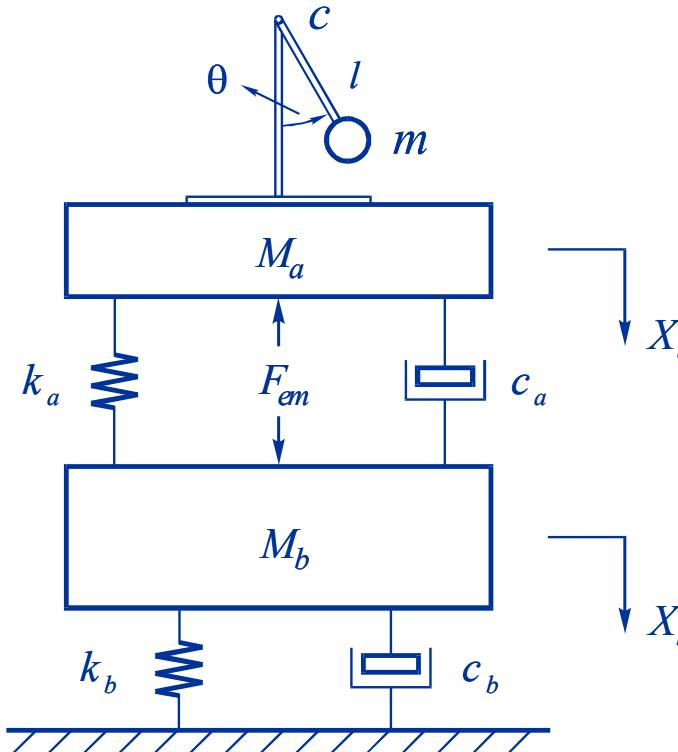
$$\frac{d}{dt}\left(\frac{\partial \mathcal{L}}{\partial \dot{q}_i}\right) - \frac{\partial \mathcal{L}}{\partial q_i} + \frac{\partial \mathcal{D}}{\partial \dot{q}_i} = Q_i$$
