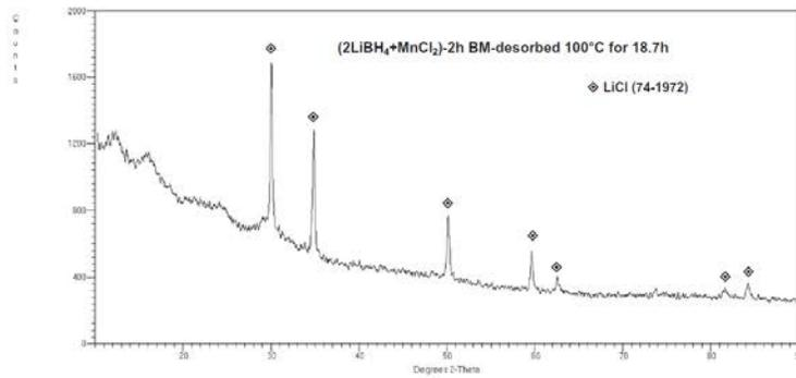
Fig. 4. XRD patterns of the synthesized nanocomposite ( $\text{Mn}(\text{BH}_4)_2 + 2\text{LiCl}$ ) after dehydrogenation at  $100^\circ\text{C}$  for 18.7 h.
