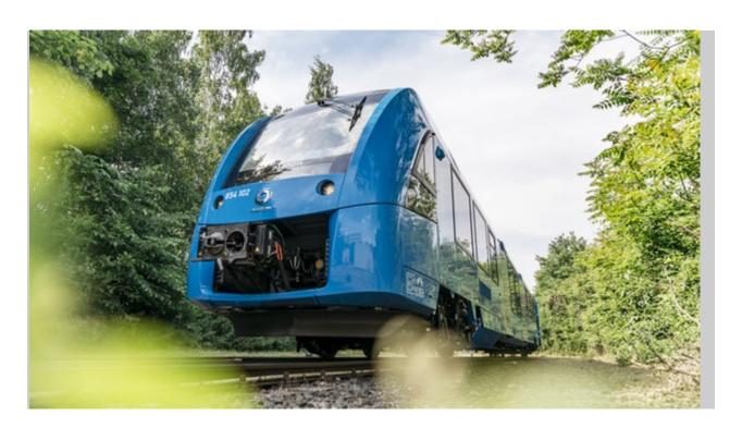
The hydrogen fuel cell-powered Coradia iLint on the move (Credit: Alstom/René Frampe)
